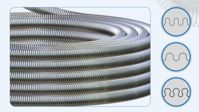
Flexible metal hoses are produced by welding a 0.15 – 0.40 mm thick stainless steel strip longitudinally under protective gas from inside and outside and then forming either mechanically or hydraulically. Mechanical forming is a four step process as can be seen below. Process called forming is necessary to shape thin sheet without being harmed. It also makes it possible to produce metal hoses in any profile without extra costs for molds.
